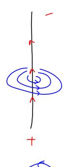
Magnetic field around a current-carrying wire.
